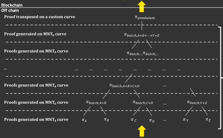
Multiple batching of proofs following the Pendulum protocol (alternation between MNT4 / MNT6 curves and final transposition on a custom curve embedding MNT6)
